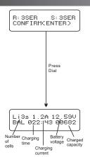
This screen displays the number of cells you set up and the processor detects. R shows the number of cells detected by the charger and S is the number of cells set by you at the previous screen. If both numbers are identical you can start charging process. If not, press button to go back to previous screen to recheck the number of cells of the battery pack before going ahead.
