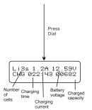
S is the number of cells set by you at the previous screen. If both numbers are identical you can start charging process. If not, press button to go back to previous screen to recheck the number of cells of the battery pack before going ahead.
