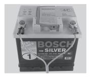
Using terminal clip attaching to car battery
