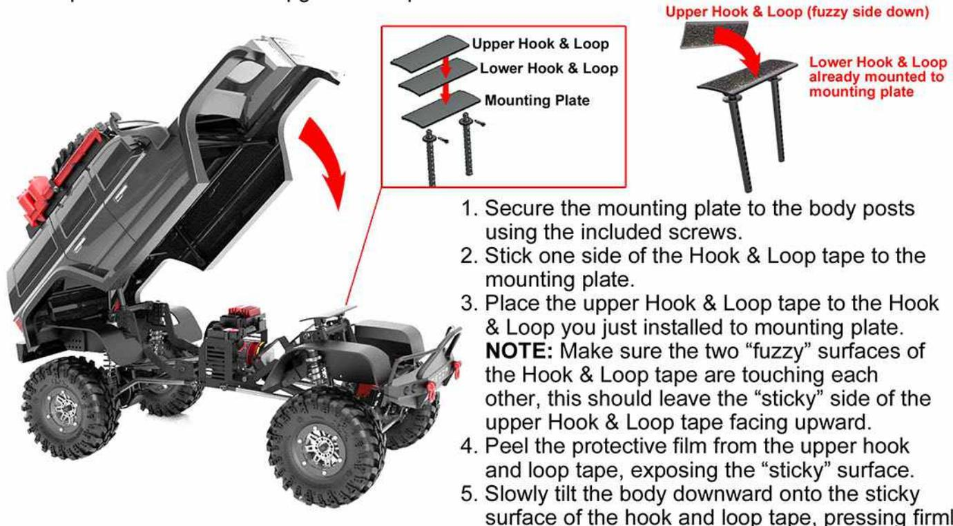
1. Secure the mounting plate to the body posts using the included screws.
