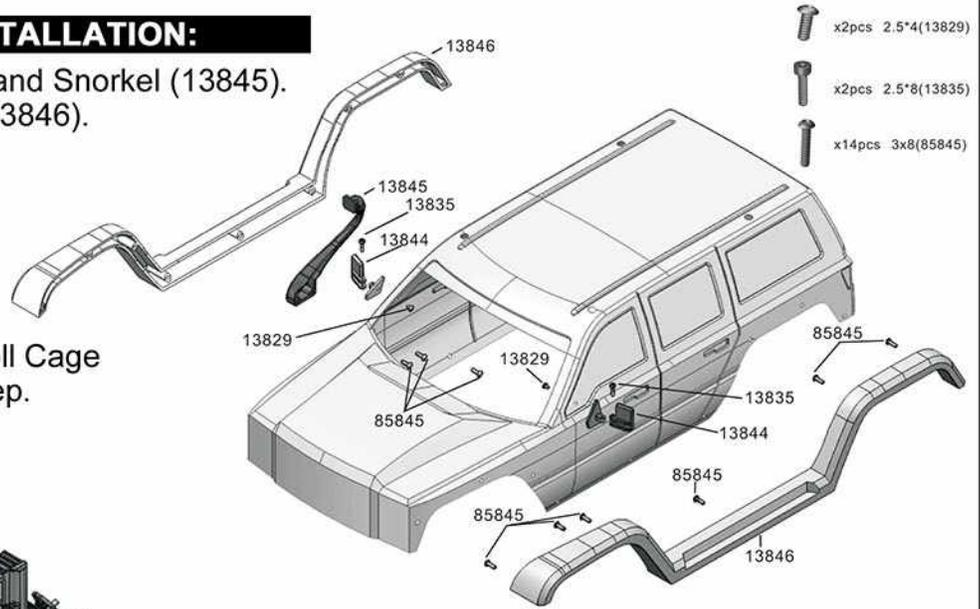
3. Insert the Roll Cage inside the body as shown.
