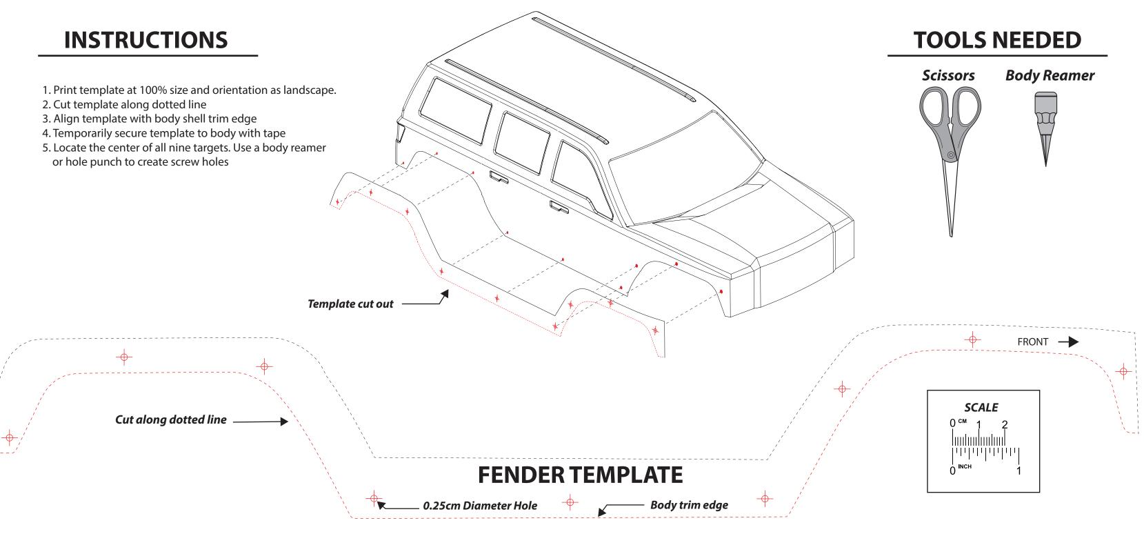
TIP: Make a small dimple in the body shell before drilling holes. Use dimples to confirm all holes are correctly aligned to the plastic fender screw holes. Once proper alignment is confirmed, drill final 0.25cm diameter holes.
