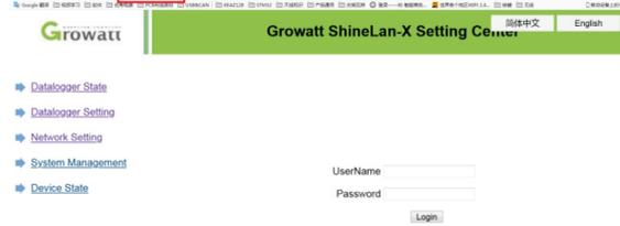
4. Enter the 'Network Setting' page, turn off the DHCP enable of the datalogger, and enter the static IP, gateway, mask, DNS. Then click to save.
