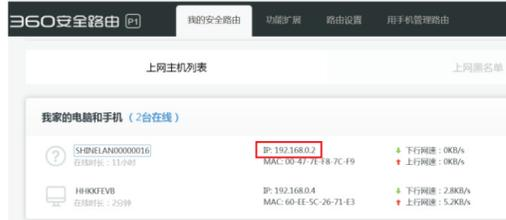
3. Open the browser, enter the dynamic IP address of the datalogger ShineLan-X in the browser address bar, and enter the built-in interface of the datalogger (account: admin, password: admin).
