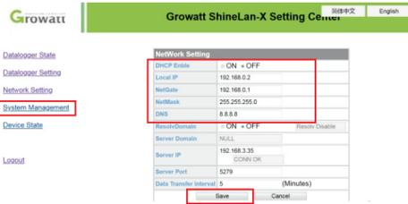
5. Enter the 'Datalogger Setting' page, enable the reboot function, and click Save. The static IP setting of the datalogger is successful.
