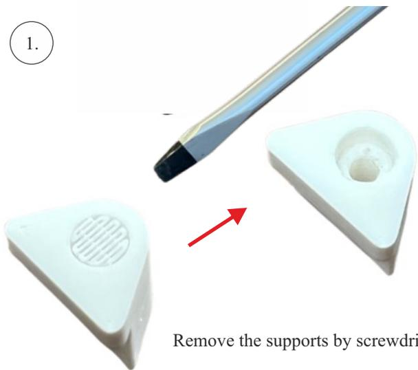
Remove the supports by screwdriver
