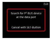
Now connect the P²-BUS device (P²-ServoBridge or P² servo) directly to the Data Port of the Royal SR2; the device is powered and read out via this port.
