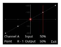
The procedure is very simple: use buttons I and II to select the point on the curve which you wish to change, then press the SET button. The servo automatically moves slowly to the corresponding point. Now you can alter the servo curve at this point using buttons I and II.
