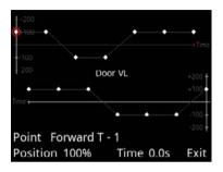
In Manual Setup you can set seven travel points in time and position for each function; forward and reverse processes are individually variable.
