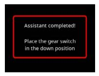
The Assistant now opens all the wheel doors and moves the undercarriage to the **Extended** position. At this point you can check the operation of the sequencer by operating the retract switch on the transmitter. If you find a problem - perhaps the pause between the undercarriage and the wheel doors is too short - you just select the Assistant again, and change the appropriate setting. There is no need to re-adjust the wheel door positions.
