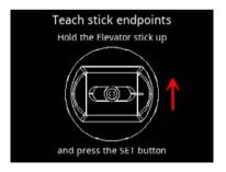
**Note:** At any time you can repeat the procedure in the Gyro menu for setting the direction of effect and the end-points. This is absolutely essential in any case if you adjust the travels or directions of effect of the primary functions while you are setting up the model.
