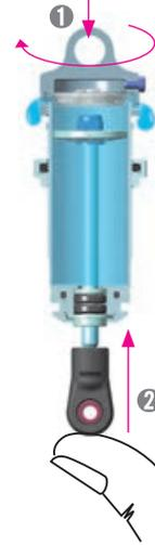
5 Gently place the shock cap assembly onto the filled shock body. Slowly compress the shock shaft towards the top of the shock body and hold in this position. Excess oil will be expelled from the shock.
