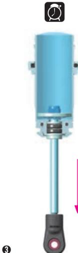
3 Orient the filled shock vertically for several minutes with the shock shaft fully extended. The remaining air bubbles will release.
