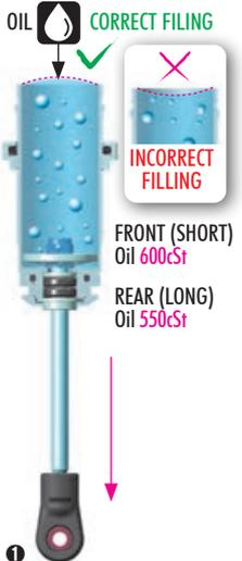
1 Extend the shock shaft completely. Fill the shock body with the shock oil.
