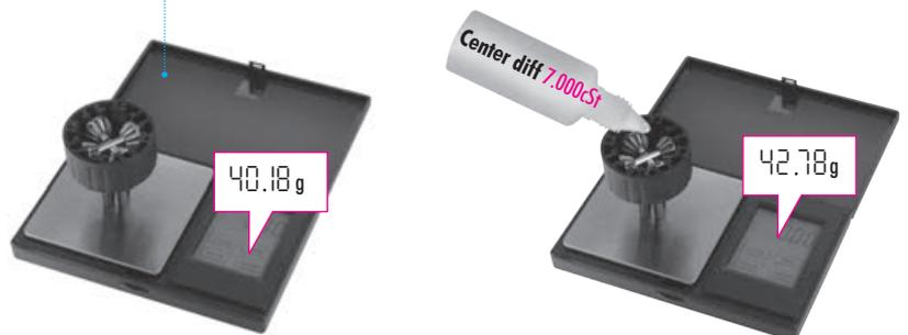
1. Put the diff (without oil) on the scale and check the weight (approximately 40.18g).
