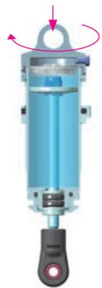
6 While still holding the shock shaft in position, fully tighten the shock cap.
