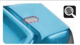
Be sure to make this rear body mount hole oval so in the case of chassis flex after a big jump the body mount will not tear up the hole.
