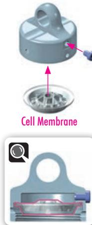
4 Install the CELL shock membrane and screw into the groove in the upper shock cap.
