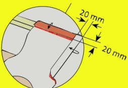
When installing the sealing strip on tiles with relief, make sure to press it down well so that it follows the roof tile's shape correctly. Make a 20-mm fold on the top part and sides to prevent water upwelling. Put spots of glue every 50cm when installing in heavy rain / high wind areas.
