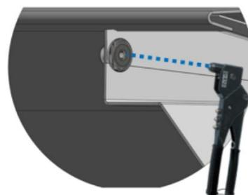
Assemble the pieces with a rivet
