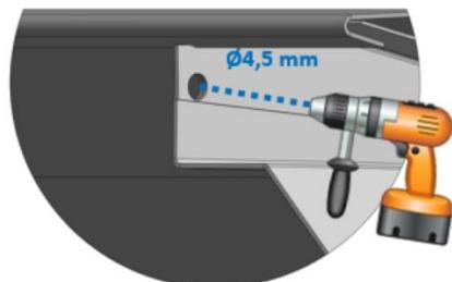
Once the height adjusted, drill the overlapped pieces with a 4,5mm drill bit
