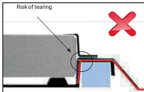
**WARNING: IN BOTH CASES, THE FLEXIBLE STRIP CAUGHT BETWEEN THE FLASHING AND THE CORRUGATION OF THE GSE PANEL MUST BE POSITIONED ON TOP OF THE CORRUGATION TO PREVENT THE RISK OF TEARING.**
