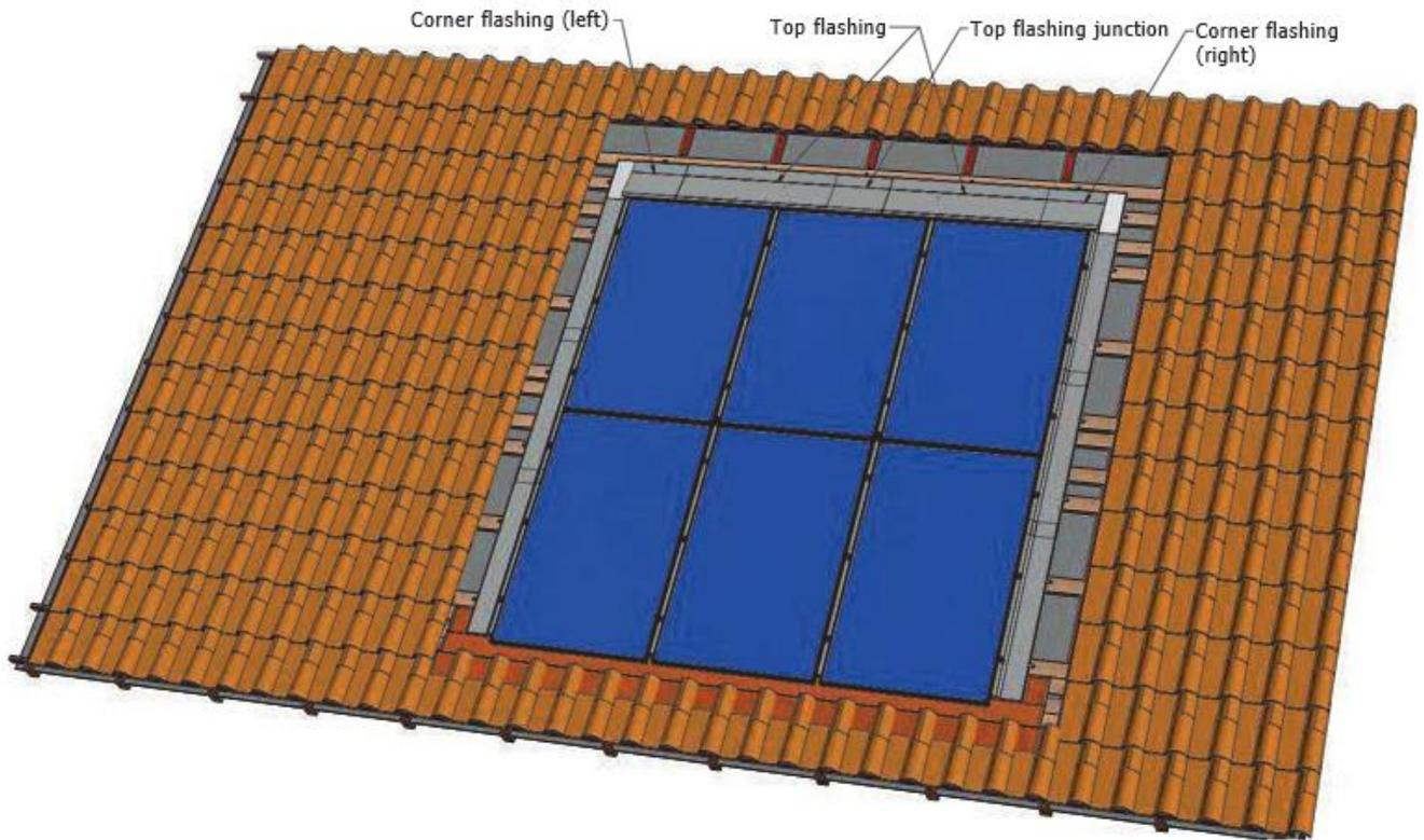
**WARNING:** THE TOP FLASHING PIECE IS DESIGNED WITH A SLOPE OF 14° TO ALLOW WATER FLOW ABOVE THE UPPER ROW OF MODULES. IT IS THEREFORE, ESSENTIAL FOR THE INSTALLER TO ENSURE THAT THE ROOF SLOPE IS SUFFICIENT TO PREVENT WATER RETENTION ACCORDING TO THE REGULATION.
