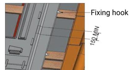
**WARNING:** FOR THE 2022 HALF-FRAMES, CUT THE ERGOT BEFORE PUTTING THE LATERAL FLASHINGS ON THE FRAMES' CORRUGATIONS
