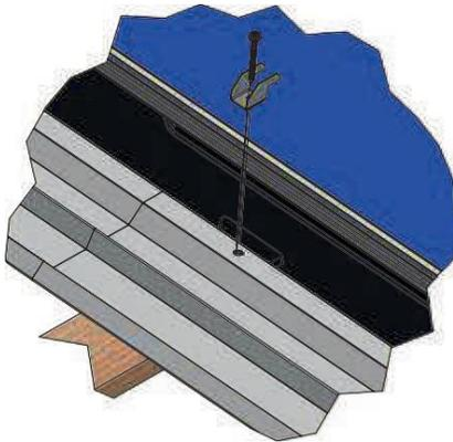
1. Unscrew the fixing clamp, remove the module and remove the edge wedges.
