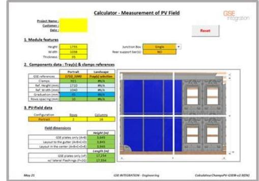
The dimensions of the PV array can be calculated using the GSE frame reference (see sections 1.4, 1.5 and 1.6 to determine the GSE frame compatible with the module):
