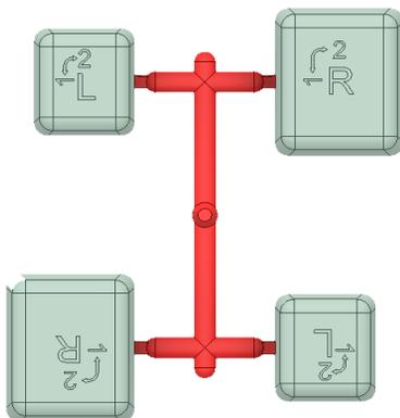
**TIP:** Mark their position on the inner surface of the frame to identify them after positioning the lateral flashings.
