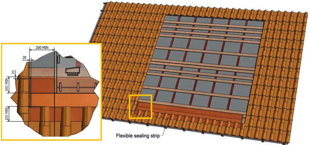
The sealing strip is laid out to link up with the bottom part of the roofing (PV array in the middle of the roofing).
