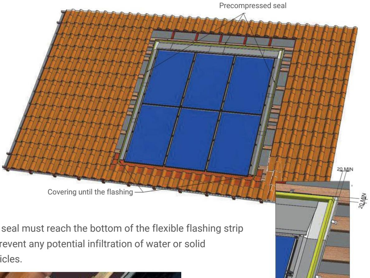
The seal must reach the bottom of the flexible flashing strip to prevent any potential infiltration of water or solid particles.
