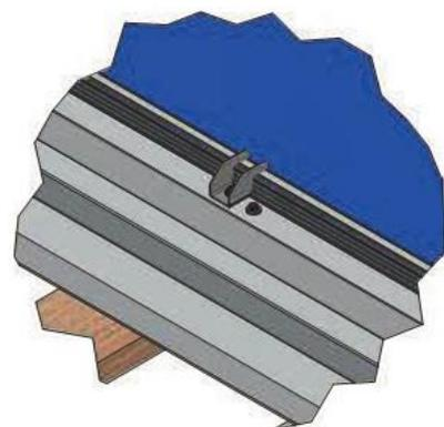
4. Place the module and attach the new assemblies (fixing clamp + EPDM foam + GSE screw).
