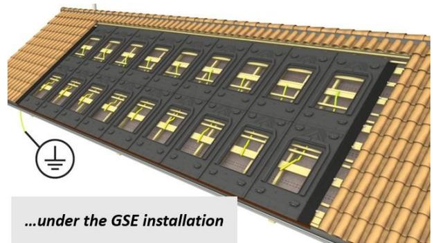
**WARNING: WHEN SETTING UP THE CABLES, MAKE SURE YOU DO NOT CREATE ANY INDUCTION LOOP, IN ACCORDANCE WITH REGULATION.**
