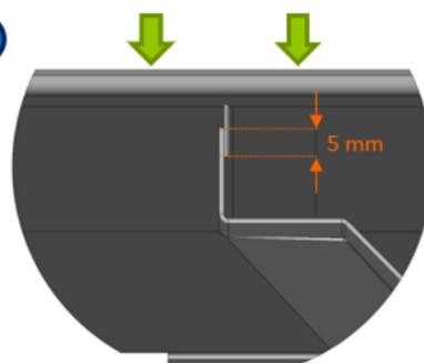
Adjust the height of the corner flashing by overlapping the two pieces
