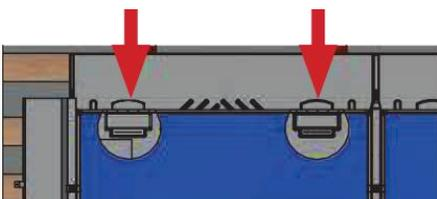
**WARNING: CHECK THAT THE MODULES ARE WELL CENTERED IN RELATION TO THE FRAME SO THAT THE GRIP OF THE CLAMPS IS THE SAME ON BOTH SIDES. THE MODULE FRAME MUST ABUT AGAINST THE UPPER PADS OF THE PANEL TO PREVENT SHIFTING.**
