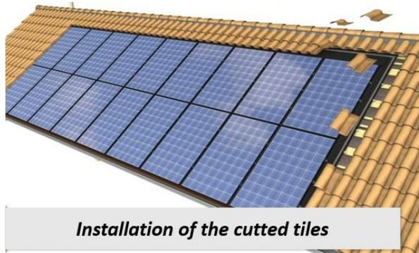
It may be necessary to cut the tiles to ensure a compliant overlap between the elements, according to roofing regulation. These elements must be attached mechanically, as described in the roofing regulation.
