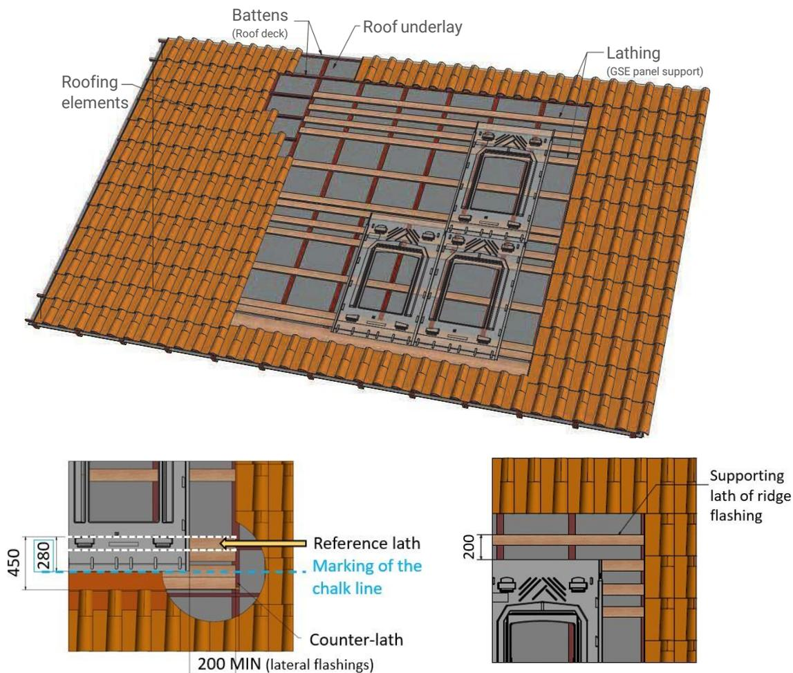
**WARNING: THE POSITION OF THE FIXING CLAMPS AND THEIR SUPPORT BATTENS MUST COMPLY WITH MODULE MANUFACTURER REQUIREMENTS.**
