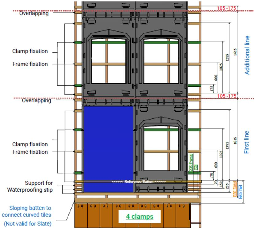
**BATTENING PLANS FOR PORTRAIT FRAMES WITH A REFERENCE HEIGHT OF 1710 MM AND 8 FIXING CLAMPS:**
