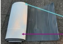
**Warning:** lay the waterproofing strip right side up
