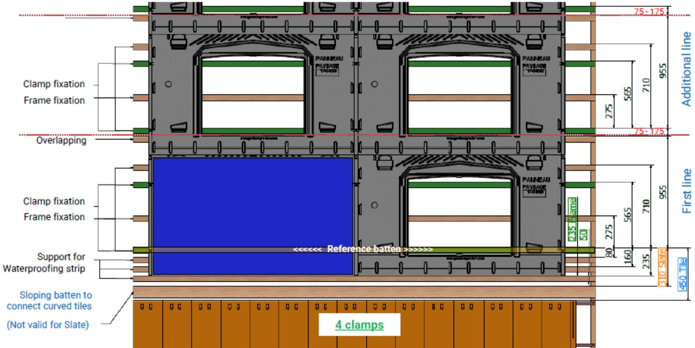
**EXAMPLE OF BATTENING PLANS FOR LANDSCAPE FRAMES WITH A REFERENCE HEIGHT OF 1020 MM AND 8 FIXING CLAMPS:**
