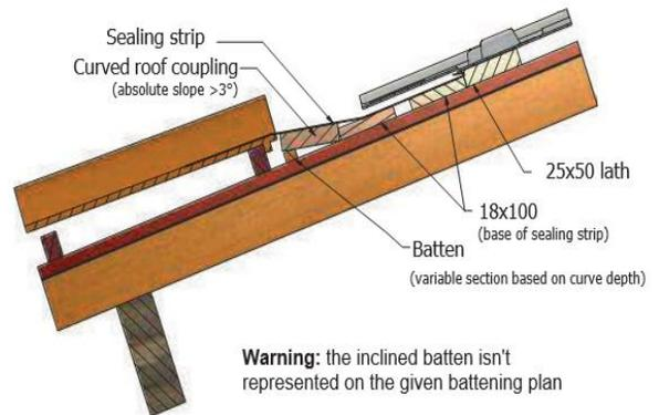
A batten is placed to fit with the thickness of the roof tile and to provide a flat base for the sealing strip.
